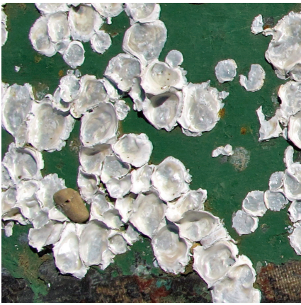
Boat bottom with anti-fouling paint and barnacles.
